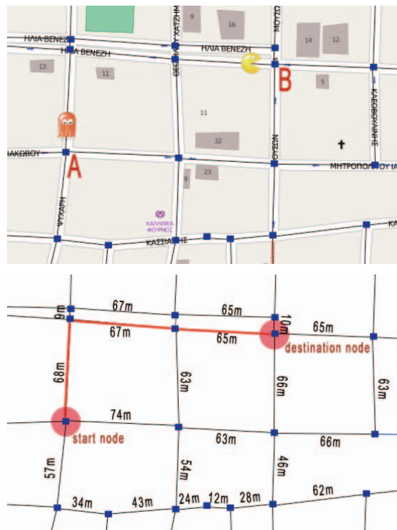
Fig. 3. (a) An example game space illustrating the extracted topology nodes; (b) shortest path derived by a directions service executing Dijkstra’s algorithm upon a graph transformation of the game space.
