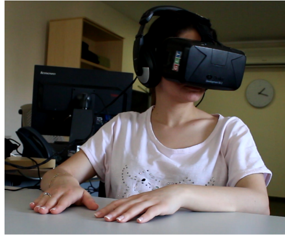
Figure 1: Participants were fitted with an HMD device for stereo display and head tracking and with headphones for stereo sound.
